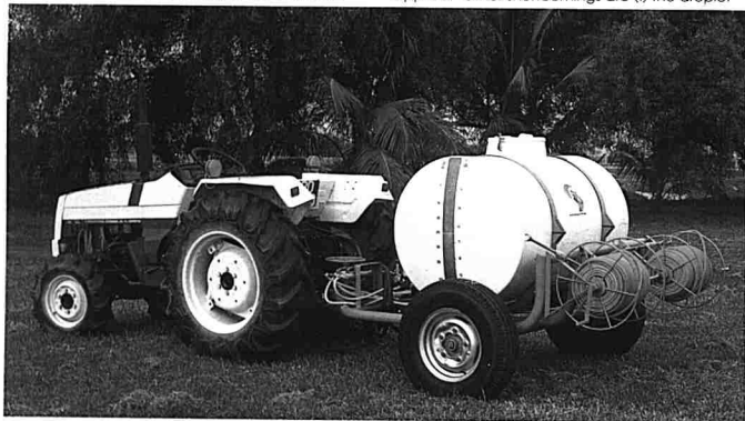
A trailer mounted mechanize spray system - The ACM SS-A1 (Courtesy of Agricultural Chemical (M) Sdn. Bhd.)
